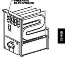
Fig. 8 - Cleaning/Inspect Openings of Primary Heat Exchangers
